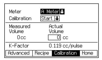
Fig. 50. Calibration Screen
